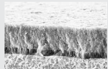
Detailansicht Feinstkornhartmetall (links) und Schichtaufbau TERAspeed (rechts). Detail of micor-grade carbide grade (left) and coating structure of TERAspeed (right).
